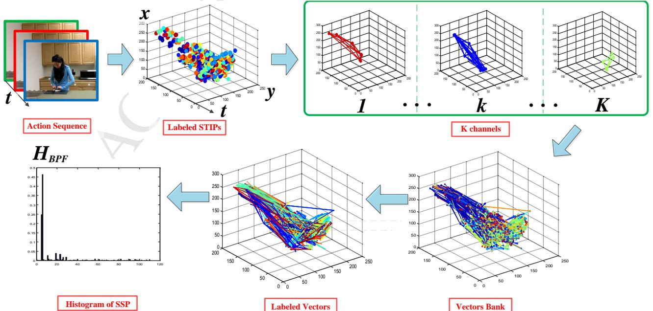
Figure 7: Flowchart of extracting SSP feature from pairwise points
