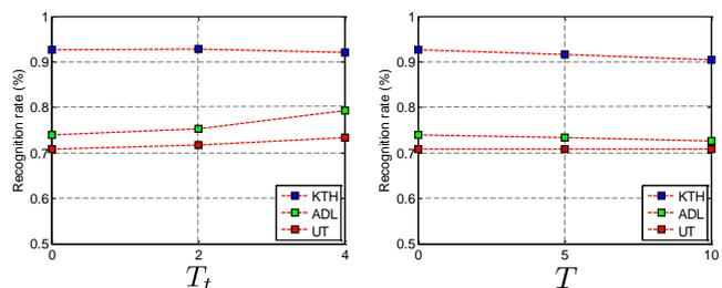
Figure 10: Classification precisions using TSP with different parameter settings.
