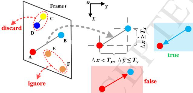
Figure 4: Direction assignment criterion for pairwise STIPs in the same frame
