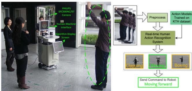
Figure 15: Applying human action recognition method to interact with robot named “Pengpeng” in a noisy environment.
